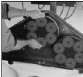
9) Move the SWOOP to where the polishing is to begin and return deck assembly to the operation position.
