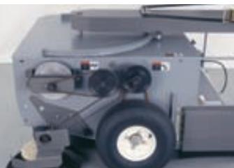
Side cover is easy to remove to adjust and change belts.
